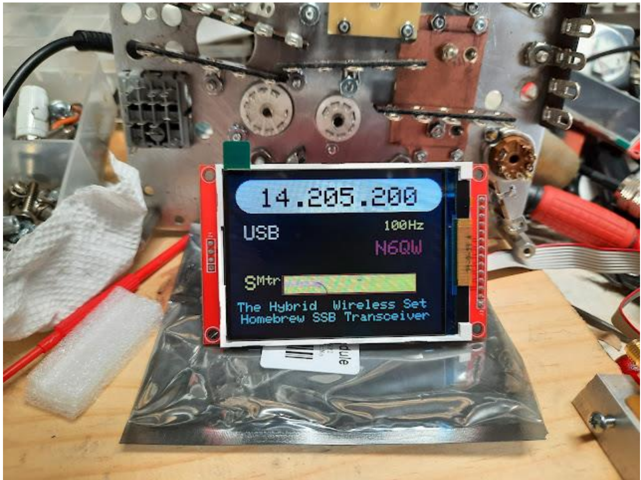
The Digital LO/BFO Used in the Wireless Set ~ An example of the Possible!
