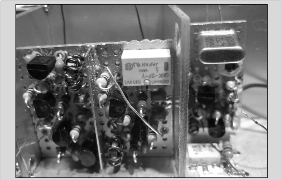
Figure 5—Bilateral amplifier and BFO photo.
